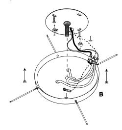
5. Secure the fixture against the mounting surface using the mounting cap **C** provided.
